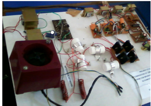
Fig.12 b. Photographic View of Hardware after connecting Z-source
